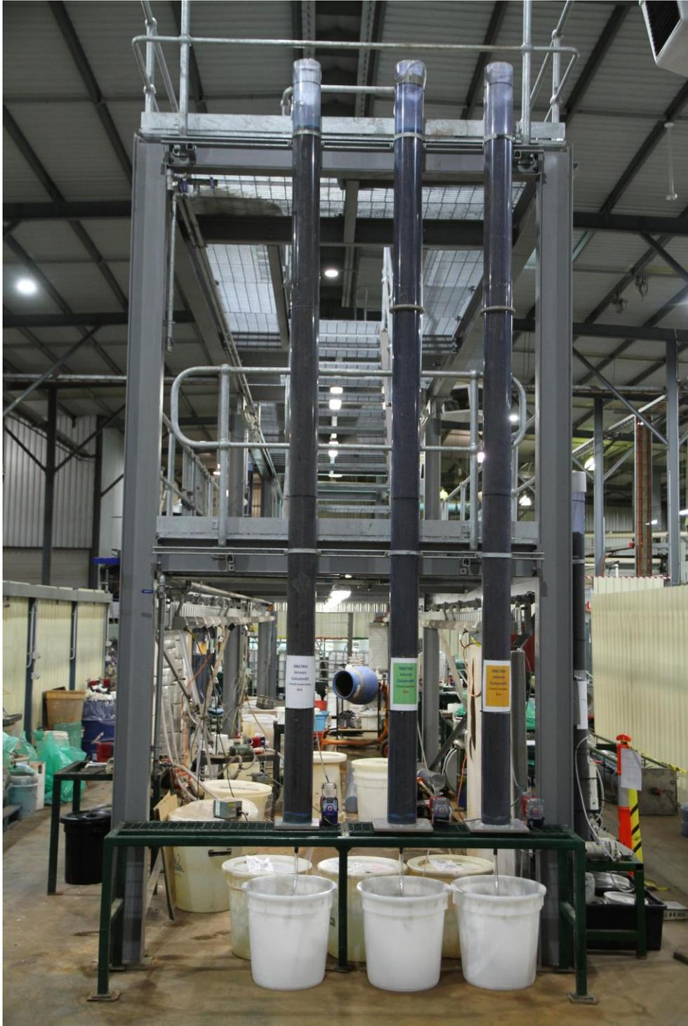
Figure 1: Jervois' 4m column samples from Nico Young being tested at SGS' laboratory in Perth.
